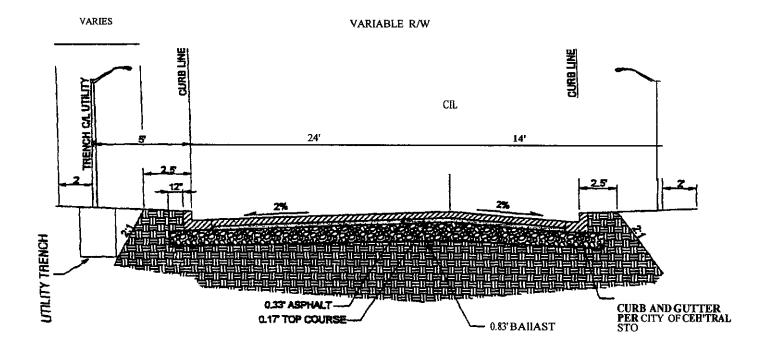
Roadway Improvements & Standards: Industrial Internal Access Road (Shown with a turn lane. Otherwise a 28 ft. curb to curb width)
